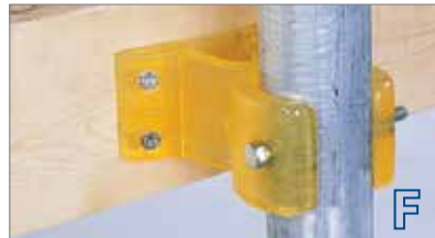
POLY PIPE STAND-OFF BRACKET Bracket attaches top of pipe to stationary docks. Fits pipe from 2.5" to 3.5" O.D.
